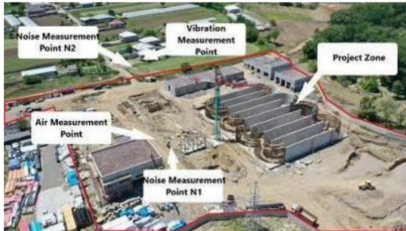
**Used Measuring Device Noise, vibration, Air Pollution under MAR-01 sub-project**
