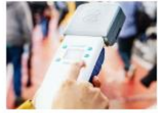
Figure 4.1.1 Air Quality Monitoring Instrument Aeroqual Sentry M8
