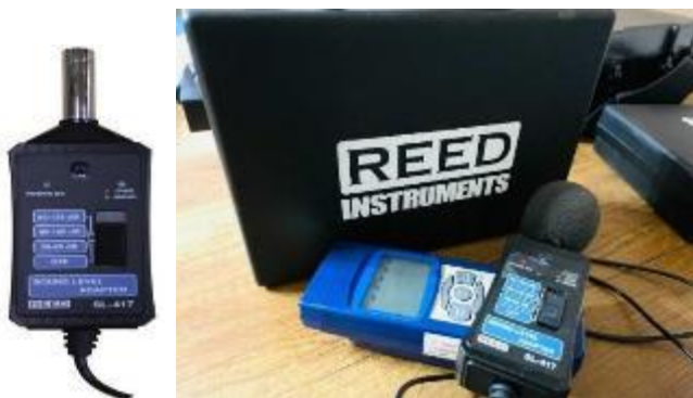
Figure 2: Noise level is determined by the REED INSTRUMENTS 9300 model adapter
