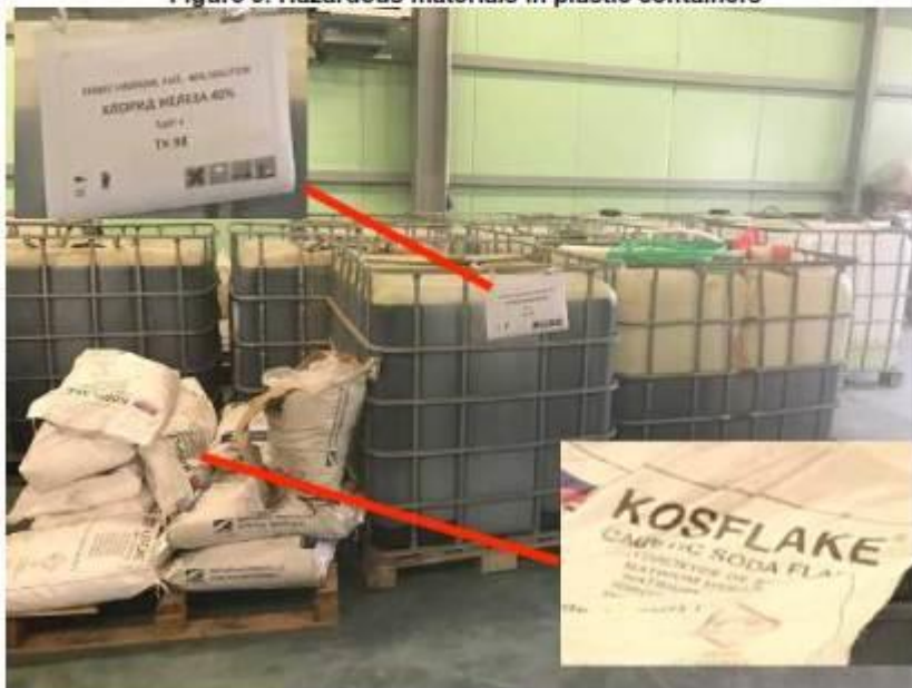
Figure 9. Hazardous materials in plastic containers
