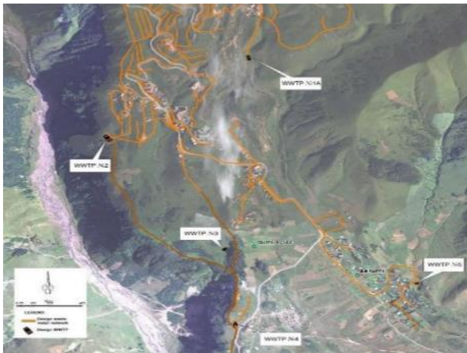
Figure 2: Design Locations of WWTPs and Approach to the Main Collectors of the New Waste water Network
