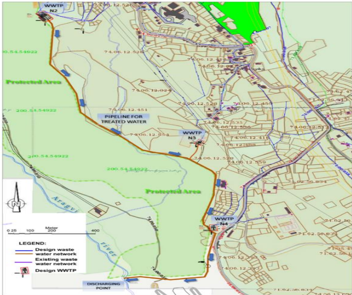
Figure 4: New Design pipeline for treated water connecting the future WWTPs #2, #3, #4 and the discharging point at the Aragvi river, bordering and outside the natural protected area.
